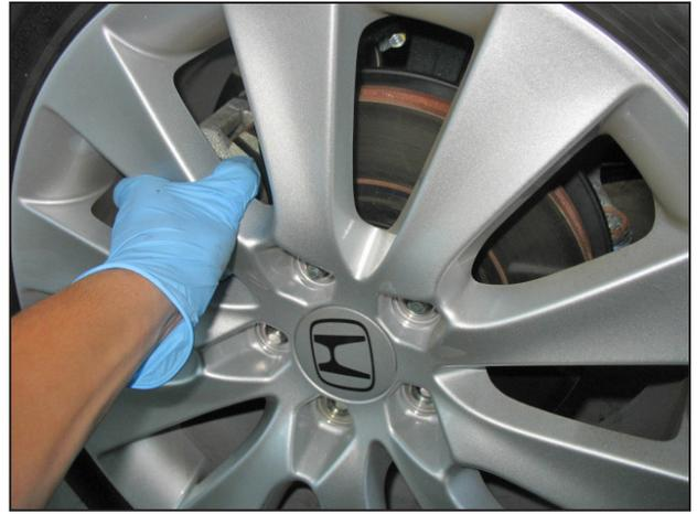
u. Install the driver side wheel using the factory torque specification (see owner's manual).
