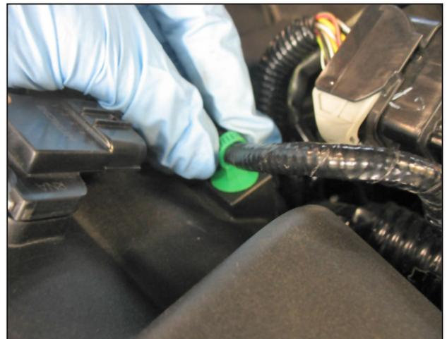
i. Remove the green clip securing the wire harness to the air box panel.
