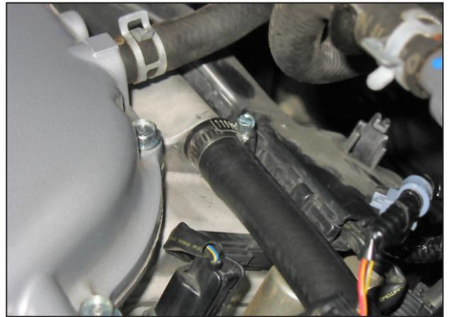
d. Insert the 1/2" hose (5-5016) onto the crank case, securing with the 1" hose clamp. Leave the other end open for now.
