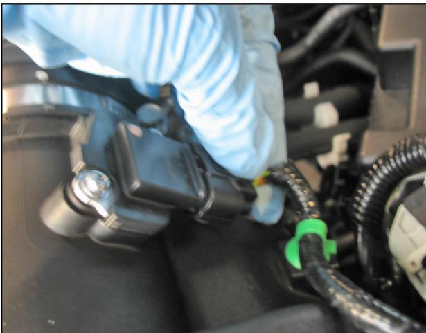
h. Unplug the wire harness connection from the MAF sensor.
